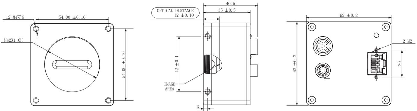
Figure1-2: CMOSIS Sensor Cameras with 62 \* 62 \* 35.3mm housing.
