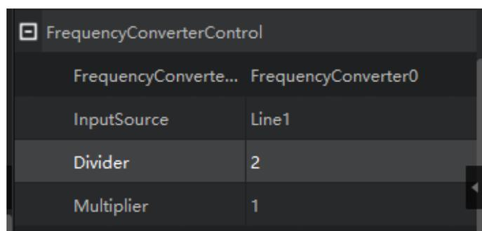
Step 4: Set a proper multiplier value (13) to increase the trigger line scan rate 26624 ( $2048 \times 13$ ). Similarly, when the image is stretched, you can adjust the divider value.
