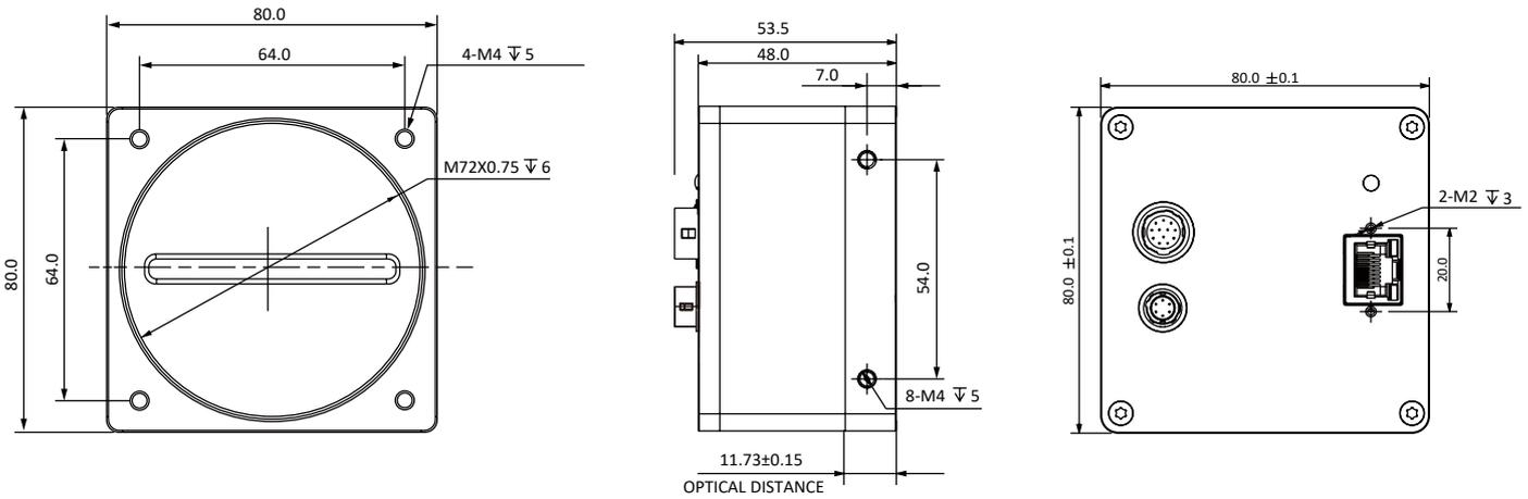
Figure1-5: 8K CL Cameras with 80 \* 80 \* 48mm housing.
