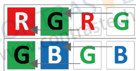
Color Camera Binning Horizontal Set to 2
