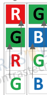
Color Camera Binning Vertical Set to 2
