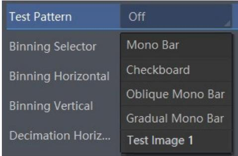
The mono camera offers 5 test patterns, including Mono Bar, Checkboard, Oblique Mono Bar, Gradual Mono Bar, and Test Image 1.
