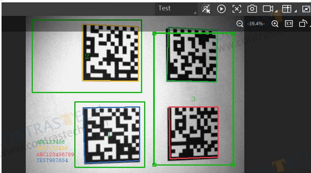
If the effect is not very good, you can adjust the focus knob (the manual focus device only) or related parameters in Image Settings area. Includes exposure time, gain, gamma, and light source parameters. At the same time, for manual focusing equipment, the focus knob on the side of the device can be manually adjusted; For devices with mechanical focus lenses, the image effect can be adjusted through the autofocus function.
