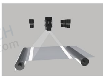
Schematic diagram of single-oblique light distribution
