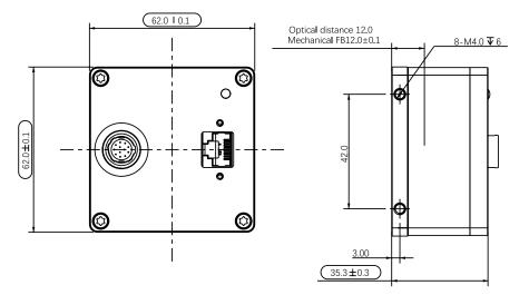
Figure1-3: Gpixel Sensor Cameras with 62 \* 62 \* 43.5mm housing.
