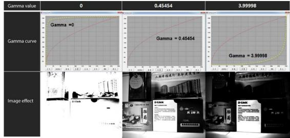
Adjust the Gamma value to make the image brightness meet the requirements.
