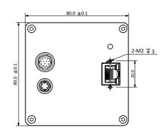
Figure1-5: 8K CL Cameras with 80 \* 80 \* 48mm housing.
