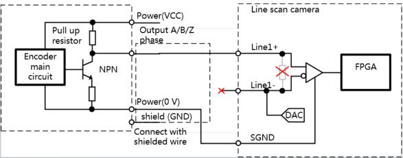
For NPN collector output, it is required to connect a pull-up resistor between the encoder power supply (VCC) and the signal cable. For PNP collector output, connect a pull-down resistor between the encoder power ground (0 V) and the signal cable. The resistance value is generally between 1–10 K, depending on the power supply voltage of the encoder. The resistance can be 1/8 W metal film in-line resistance. See Table below for the recommended values.
